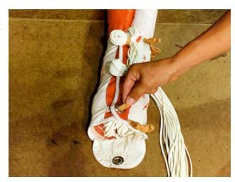
G. CLOSE THE END FLAP OVER BOTH OF THE SIDE FLAPS USING A STOW NO MORE THAN 1 1/2" LONG.
