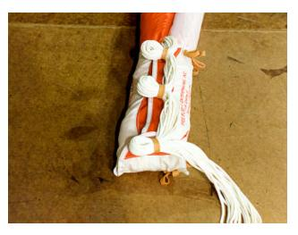
H. FINISH STOWING THE REMAINDER OF THE SUSPENSION LINES. USE STOWS NO MORE THAN 1 1/2" LONG. COMPLETE THE PACKING PROCEDURES USING THE INSTRUCTIONS PROVIDED BY THE MANUFACTURER OF THE CONTAINER AND HARNESS.
