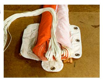
E. FORM A LOOP OF SUSPENSION LINES, NO MORE THAN 1 1/2" LONG. CLOSE THE DIAPER, STARTING WITH THE TOP GROMMET. THEN CLOSE THE CENTER GROMMET.
