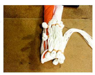
I. IT IS MANDATORY THAT THE PILOT CHUTE BRIDLE BE INSTALLED THROUGH BOTH OF THE POSITIONING LOOPS ON TWO VENT LINES AND AROUND ALL OF THE OTHER VENT LINES. IT MUST BE SECURED WITH EITHER A BOWLINE KNOT OR STITCHING AT LEAST EQUAL TO THE STRENGTH OF THE BRIDLE MATERIAL. IT MUST HAVE A LOOP ADEQUATE TO PREVENT THE BRIDLE FROM TIGHTENING ON THE VENT LINES.
