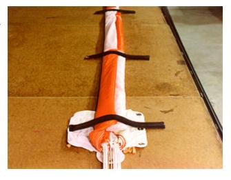
D. PULLING THE CONTAINER TOWARDS THE CANOPY, FORM A LOOP OF SUSPENSION LINES ABOVE THE TOP OF THE DIAPER. LEAVE ENOUGH ROOM TO CLOSE THE DIAPER.
